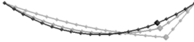
Figure 2. Tension structure where the mass of one node has been increased. The black outline shows the catenary configuration where all nodal masses are equal. The grey shows the change in shape.
